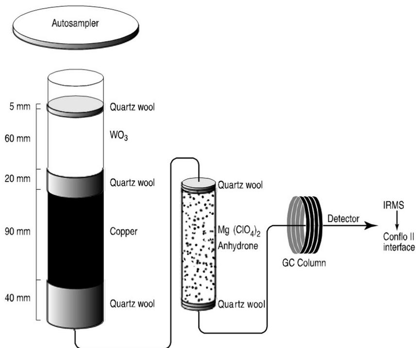
**Figure 1.** Diagram of the Carlo Erba Instruments NC 2500 (CE NC 2500) elemental analyzer (used with permission of Thermo Electron Co.).
